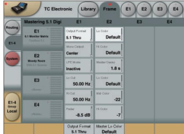
If "no Lock" is achieved or "Sample Slip" situations occur this will be indicated via the small red dot in top of the Frame Tab.
