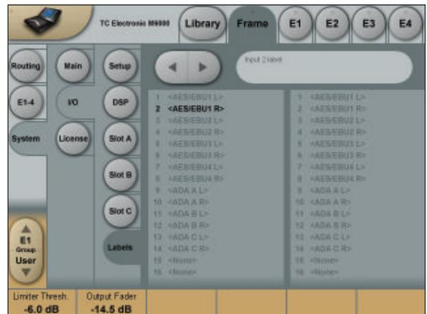
All physical Inputs and Outputs can be named/renamed. Enter the Titles page by pressing the tabs System and Titles. Press any of the 16 Inputs/Outputs and the Naming display will pop up. Enter adequate name for the Input/Output and press **Enter**.
